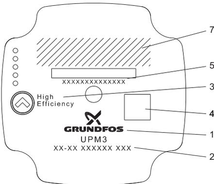
Fig. 7 Nameplate: customised layout
