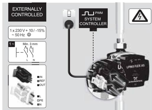
Fig. 60 Control box with FCI connection
