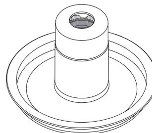
Fig. 35 Rotor can with bearing holder and ceramic bearing
