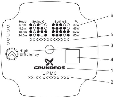
Fig. 6 Nameplate: Grundfos with setting indication
