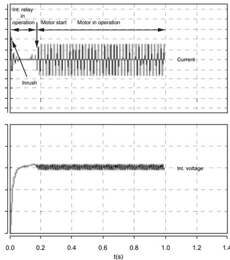
Fig. 56 Example: UPM3 with internal inrush relay
