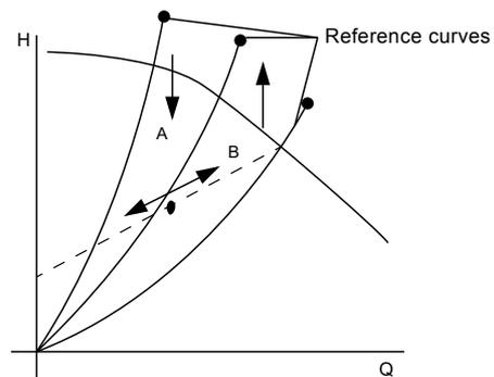
Fig. 29 Duty point on selected proportional pressure curve
