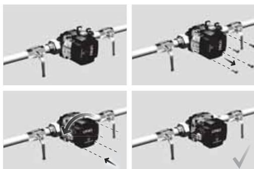
Fig. 50 Changing the control box position
