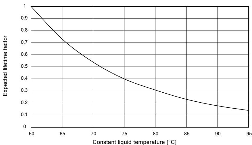
**Fig. 47** Diagram temperature/expected lifetime for PA 6.6 30 % GF
