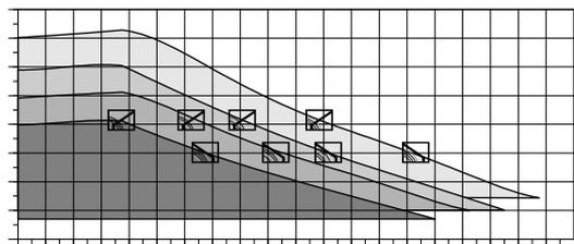
Fig. 22 UPM3 FLEX/HYBRID control modes with pump curves
