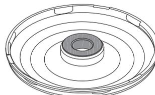
Fig. 40 Bearing plate with ceramic bearing
