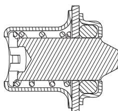
Fig. 37 Sectional drawing of deblocking device
