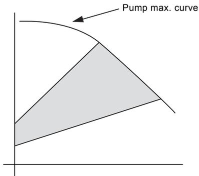
Fig. 26 Proportional pressure  $AUTO_{ADAPT}$  operation area
