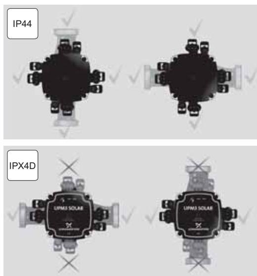
Fig. 49 Control box positions
