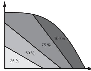
Fig. 18 Operation area according to performance load
