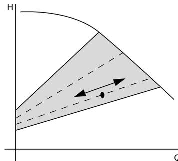
Fig. 30 New lower proportional pressure curve
