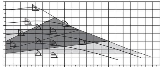
Fig. 21 UPM3 AUTO/HYBRID control modes with pump curves
