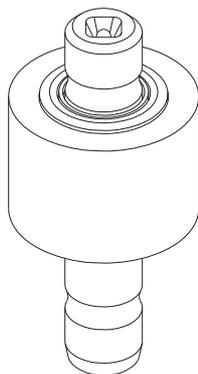
Fig. 38 Shaft with rotor
