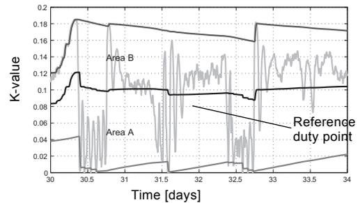
Fig. 28  $K_{sys}$ -values logged for the system analyser
