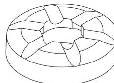
Fig. 39 Thrust bearing
